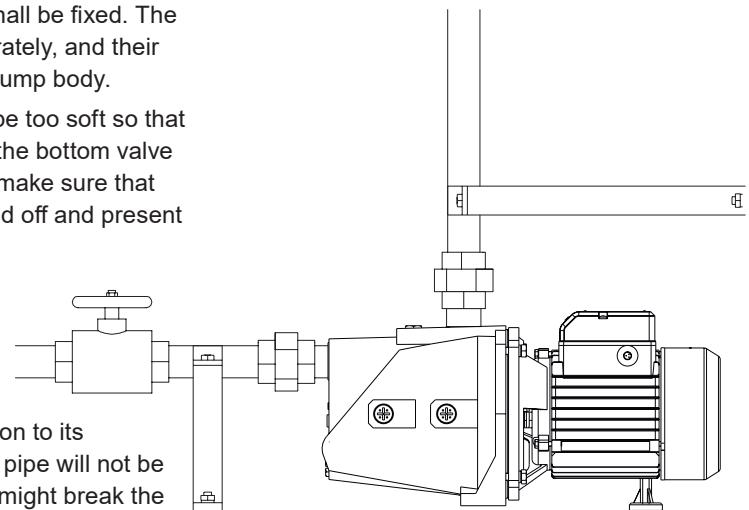
3. Connect the outlet pipe firmly to prevent water from splashing on the motor and hence causing electrical leakage of the electric pump. When a rubber pipe is used, pay attention to its temperature resistance limit to ensure that the pipe will not be deformed by heat, because such deformation might break the pipe and hence cause water leakage.
