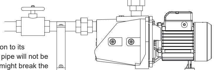
4. After connecting the inlet pipe to the inlet of the electric pump, please make sure that the end of the inlet pipe, where the bottom valve and the strainer are located, is submerged in water. To guarantee reliable operation of the electric pump, please use an effective strainer with the bottom valve, which must be more than 30cm away from the water bottom, for the purpose of preventing sludge or impurities being absorbed to the pump chamber and hence affecting the operation of the pump.
