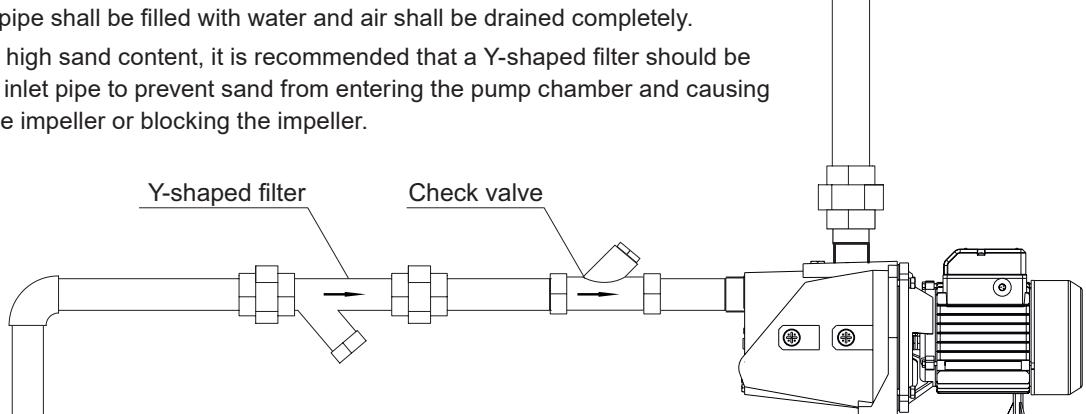
2. Prior to the use of the electric pump, please carry out a test run, the duration of which shall not exceed 10s, as long-time dry run will damage the mechanical seal. In case of a three-phase pump, please check whether the rotational direction is the same as the rotation marking. If the rotating direction of the electric pump is reversed, immediately cut off the power supply and exchange any two phases of the three-phase pump.
