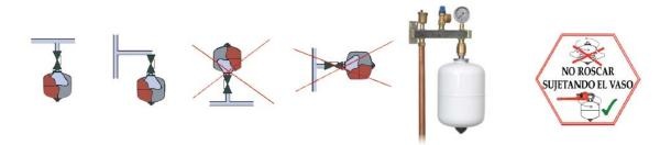
Make sure the hoses and couplings are tight and the working temperature or pressure for which is designed the expansion tank is never exceeded. Under no circumstances exceed the maximum pressure indicated on the label of the expansion vessel. The expansion tank could explode.
